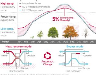
% This function is operated with 'Auto' mode by wired remote control.
