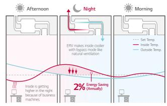
% This function is operated with 'Night Time Free Cooling' on remote controller. (with MULTI V only) % Energy saving ratio can be differed by weather condition. \* Test Condition
